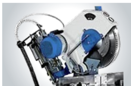
Oil-pneumatic feed of head
