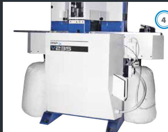
Jet of two dust collecting unit Dust collecting unit for each dust hose: Ø 80 mm Dust collecting speed: 20 m/sec Air volume each dust hose: 320 m3/h (for V235 e V235FNC)
