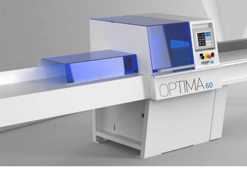
The **OPTIMA 60** is a Push-Feed Optimizing and Defecting Cut-Off Saw. It is fitted with the last generation CNC, with adjustable 10.4" Touch Screen display, combines reliability, ease of use and always maintains the ergonomic position of the operator.
