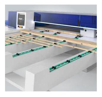
Front loader with ramps, of new design, more functional and ergonomic. Available in a variety of sizes and ramps configurations.
