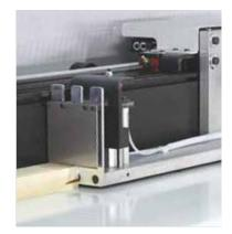
A vertical tail clamp fitted on the pusher, allows for feeding speeds of 120 m/min. while ensuring very precise cutting tolerances of +/- 0.15 mm.
