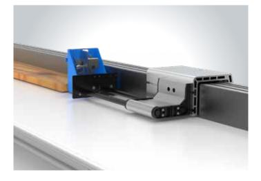
A vertical tail clamp fitted on the pusher, allows for feeding speeds of 60 m/min. while ensuring very precise cutting tolerances of +/- 0.15 mm.
